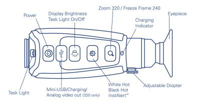
**Power Button** – Ocean Scout<sup>™</sup> has three power states: On, Off, & Auto Shutdown.
